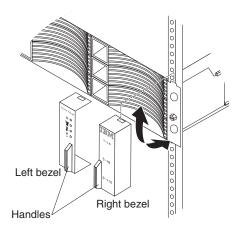
Figure 57. Removing the bezels
